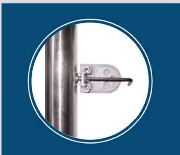
Step 4 Screw button head cap screw into blind rivet nut through glass clamp to fix half of glass clamp to post
